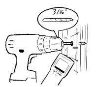
2 Pre-drill wall studs with a 3/16" bit.
