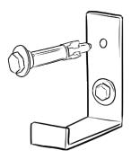
2 Install brackets with special masonry bolts.
